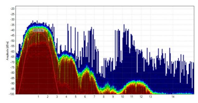
As 802.11b becomes less popular, this signature is becoming less common, but it's good to be familiar with it. This **curve shape with lobes on each side** is made by an **802.11b** network, or any 802.11g/n network running at legacy data rates like 1, 5.5, or 11 mbps. An 802.11g or 802.11n network will fall back to this shape from time to time, or when idling. To prevent this, legacy data rates can be disabled, which will improve network performance.
