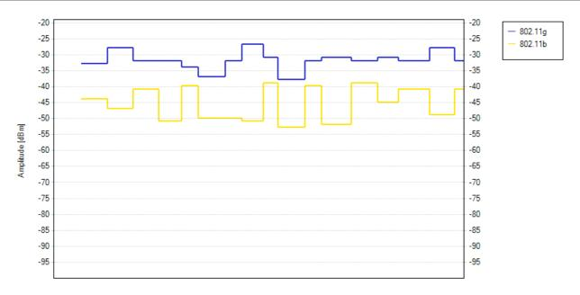
The **Networks Graph** represents Wi-Fi signal strength over time, using data collected from the computer's Wi-Fi card. The signal strength represents amplitude levels of transmit beacons that were received by the card. Drops in signal strength indicate poor coverage, and can be referenced against the Density and Waterfall views to determine if interference is the problem.
