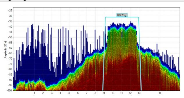
The Density View maps and displays how often a frequency/amplitude point is being used. The less trafficked frequency ranges will appear more transparent. The colors represent amplitude height with reds indicating higher signals and darker blues lower power levels. An important feature of this view is that it picks up device-specific signatures which enables analysis of what types of electronics are emitting RF energy in the area.
