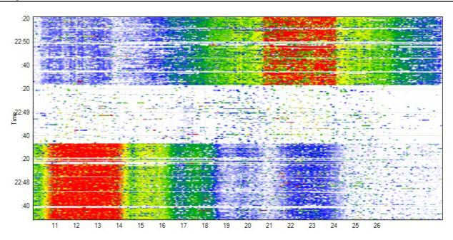
The Waterfall Graph shows amplitude over time for each frequency in the in the band, much like a seismometer graphs earthquakes over time. The colors represent power levels in the spectrum with dark blue as low, and bright red as higher amplitude levels - much like a Doppler radar weather map.
