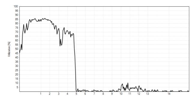
Utilization measures the percentage of activity above a defined amplitude threshold. Utilization is similar to airtime usage and duty cycle. The Utilization Graph gives more exact representations of utilization in the spectrum than the Density View's approximations.
